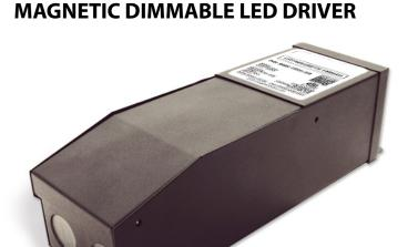
KLUS - MD-150-12 is the most compact LED driver on the market with a magnetic transformer core. It is equipped with two auto-reset breakers, one on the input and one on the output, which protect both the load and driver. The driver is encased in a coated metal box that includes 2 knock-outs, one on each side, to enable easy installation that complies with electrical code requirements.
